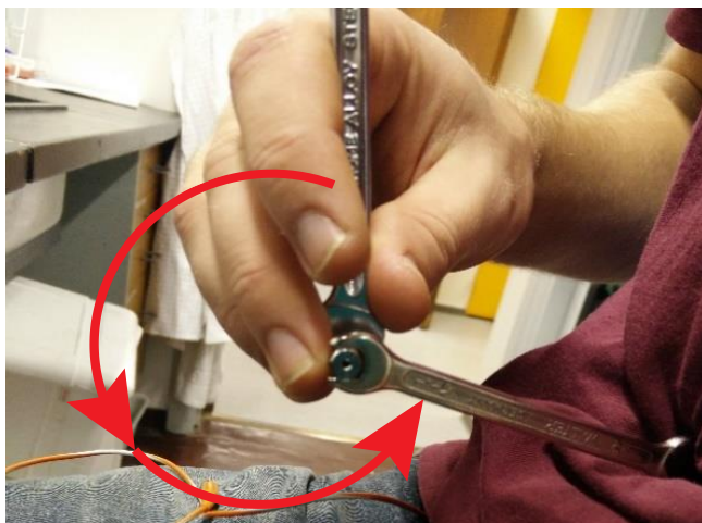
Figure 9. The red arrows indicate the amount of tightening that should be sufficient for fitting the ferrule without blocking the PEEK-tubing
