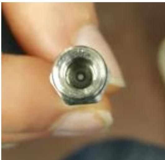
Figure 6: Notice the neat white circle. This indicates the tefzel column has been packed with beads
